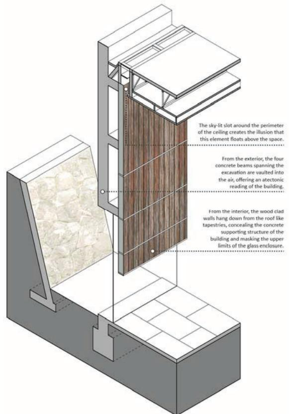
Fig. 9. Section of the Chapel del Retiro by Undurraga Devés
