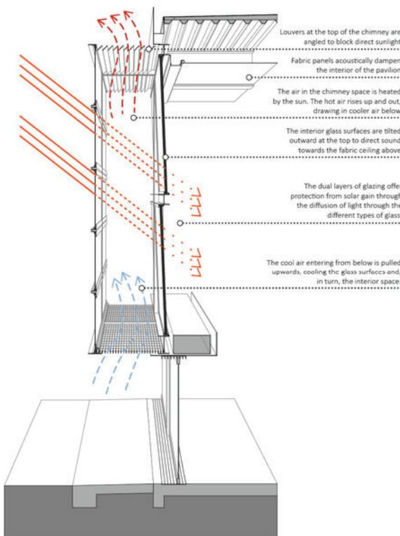
Fig. 6. Wall section of the Prayer Pavilion of Light by Debartolo Architects
