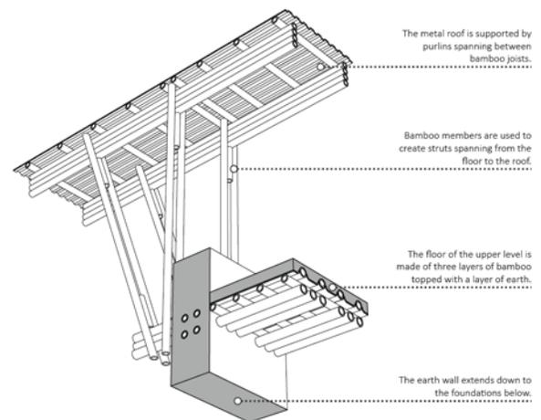
Fig. 5. Construction detail of the METI Handmade School by Anna Heringer
