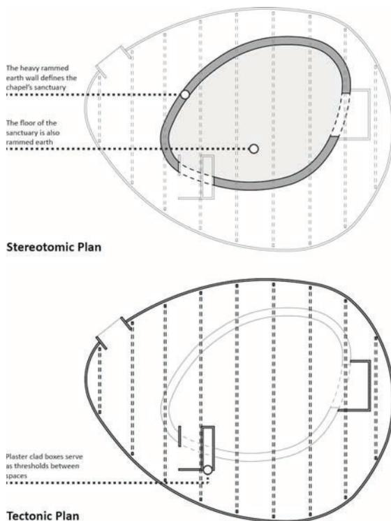
Fig. 4. Stereotomic and Tectonic plans of the Chapel of Reconciliation by Reitermann and Sassenroth.
