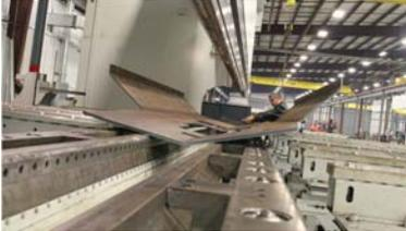
LVD 2,000 TON – 40 FT BENDING SOLUTION
