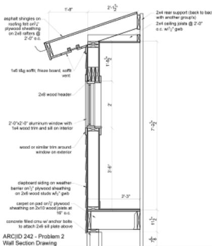
Figure 1: Building Technology I - Proposed Wall Section Drawing
